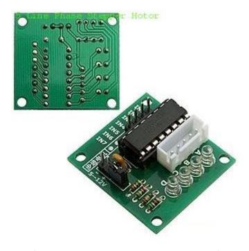
the features of four- wire five- phase stepper motor driving board: use ULN2003 high power Darlington chip to drive stepper motor driver; B, C, A, D LEDs indicate the state of the working four- phase stepper motor; set with the standard interface of stepping motor which can be directly inserted in the use.
